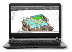
At the press of a button the polygons are created, surface areas calculated and the room information blocks created. Visualizations (e.g. different room hatches for each type of room use) are likewise automatically created. The area data can be exported in different ways, e.g. to text tables or directly to databases (for example to a CAFM system).
