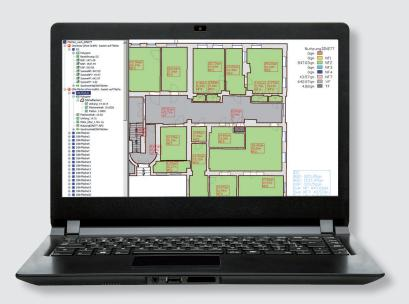
A TachyCAD surveyed floor plan. Physical data to each individual room, such as floor area and volume are automatically calculated. Recorded attribute data can be assigned to the individual rooms.
